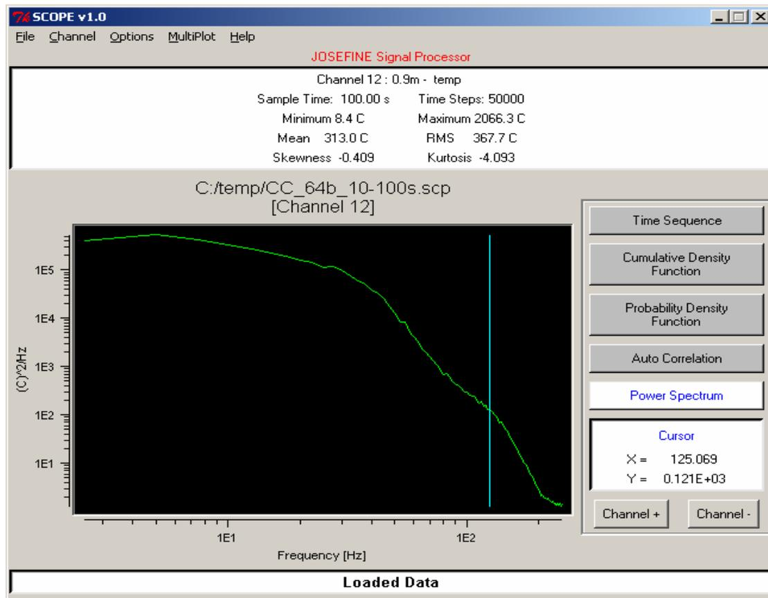
**Figure 8. Temperature spectrum determined from transient centreline temperature predictions from FDS [Welch (12)]**
