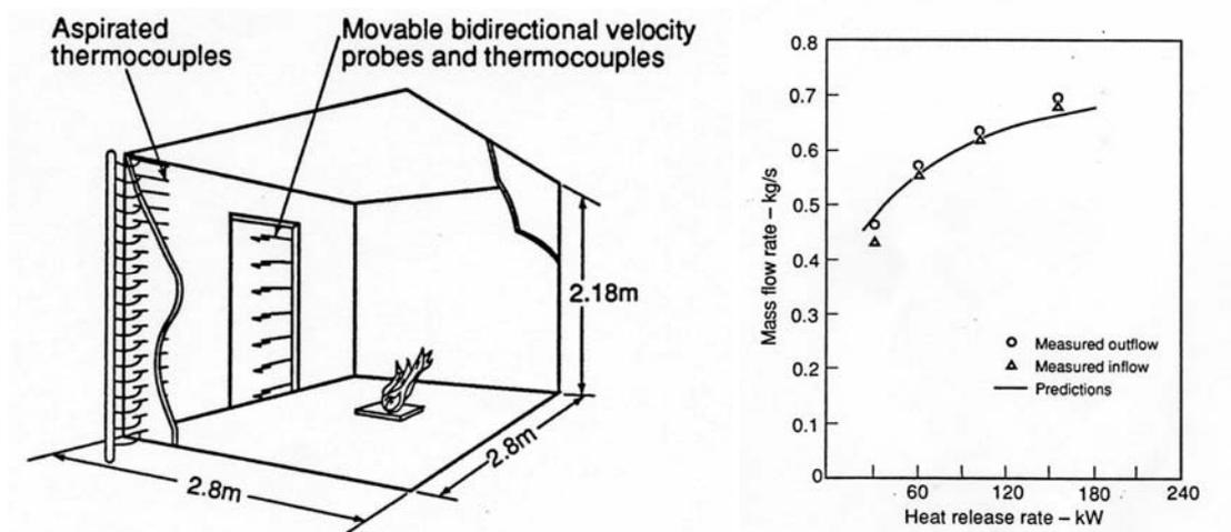
*Figure 4. Early comparison of CFD predictions of mass flow rates with measurements [Cox (14)]*
