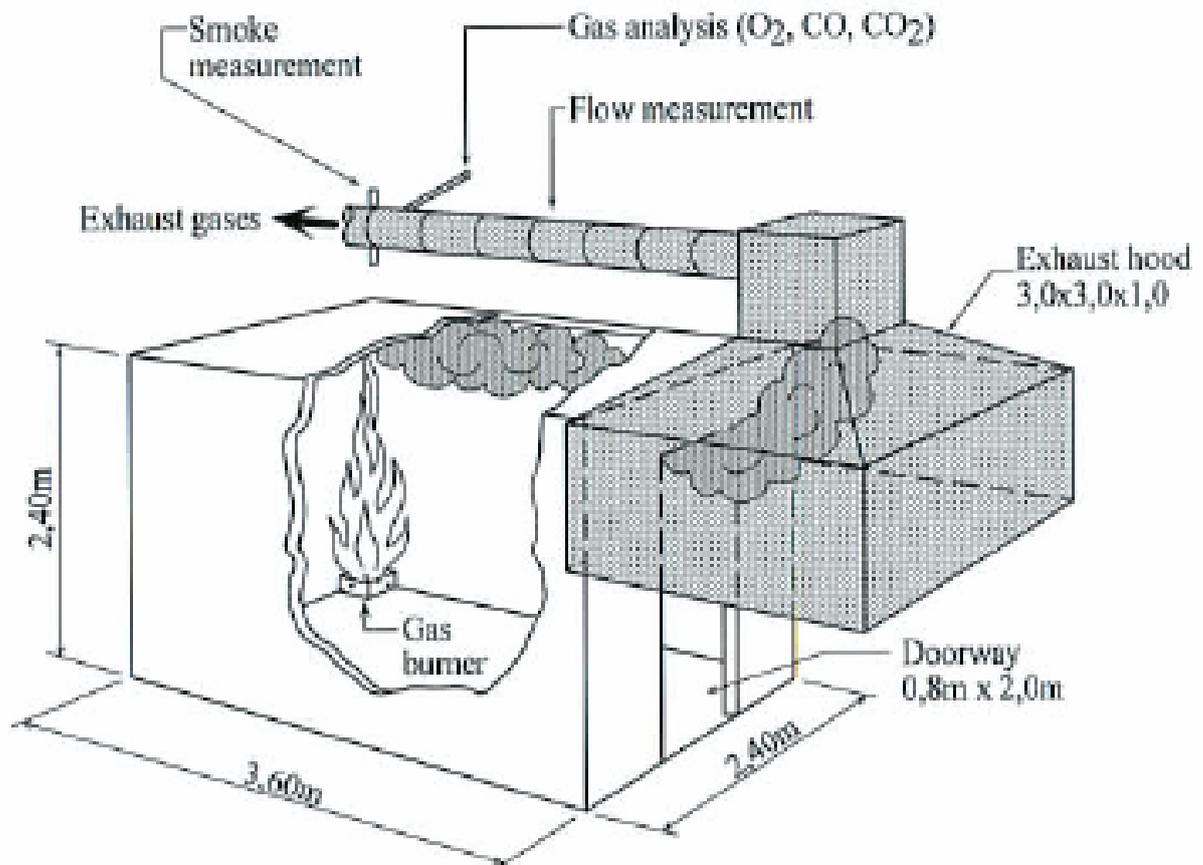
Figure 2. The ISO 9705 Room Corner test
