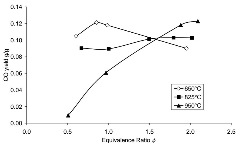
Fig. 6 Variation of CO yield with temperature and equivalence ratio for glass fibre reinforced PA6 containing brominated flame retardant.
