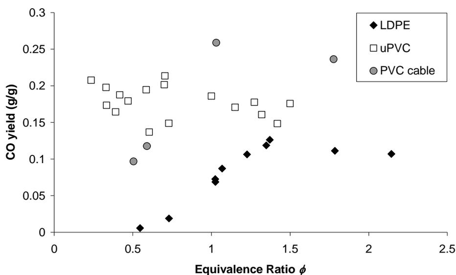
Fig. 3 Variation of CO yield for LDPE, unplasticised PVC and PVC containing plasticizer and chalk.
