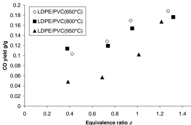
Fig. 5 CO yield of LDPE/PVC mixture at 650, 800 and 950°C.
