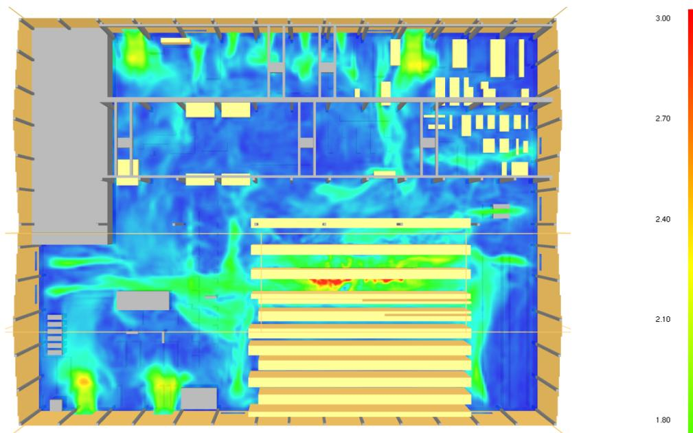
Figure 6 (a). Air velocity at 1200 s
