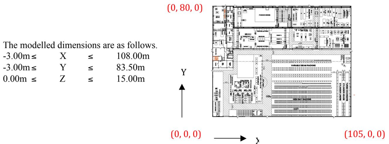
Figure 4. Model orientation and slice file co-ordinates
