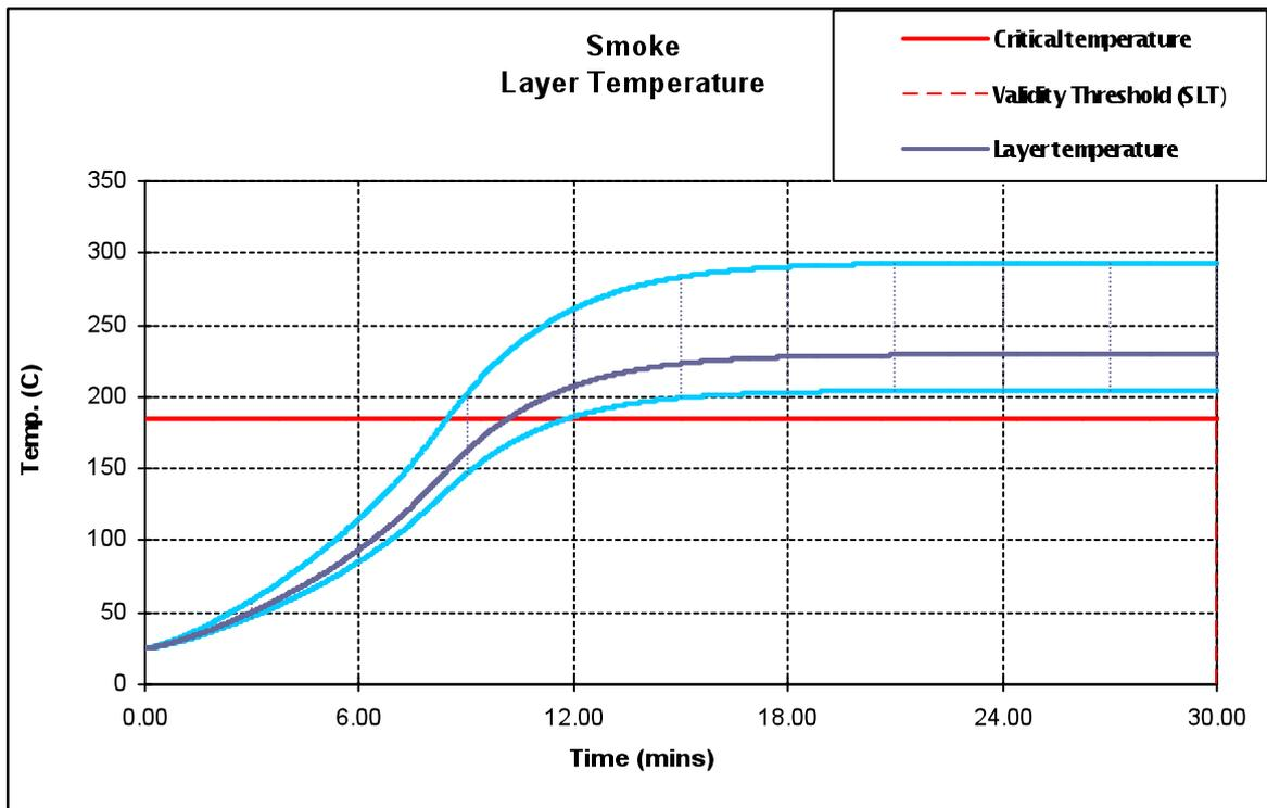
Figure 3 (b). Smoke layer temperature, Scenario 2
