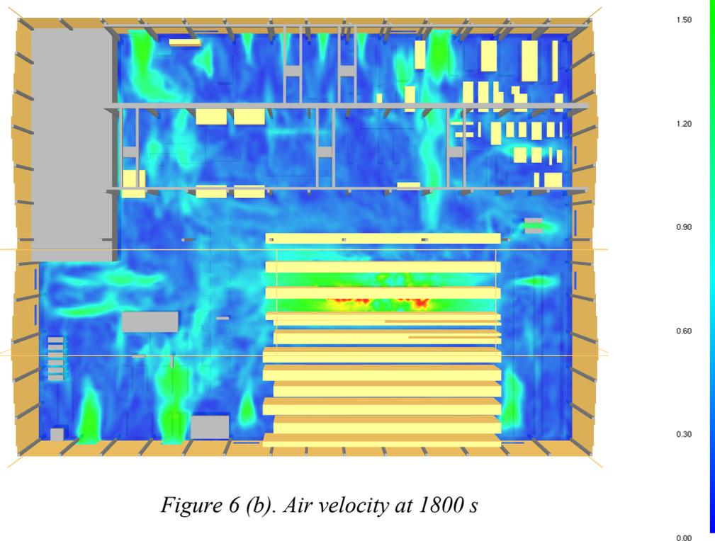
Figure 6 (b). Air velocity at 1800 s
