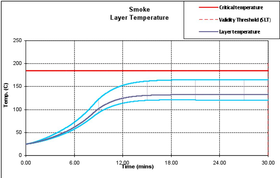
Figure 2 (b). Smoke layer temperature, Scenario 1
