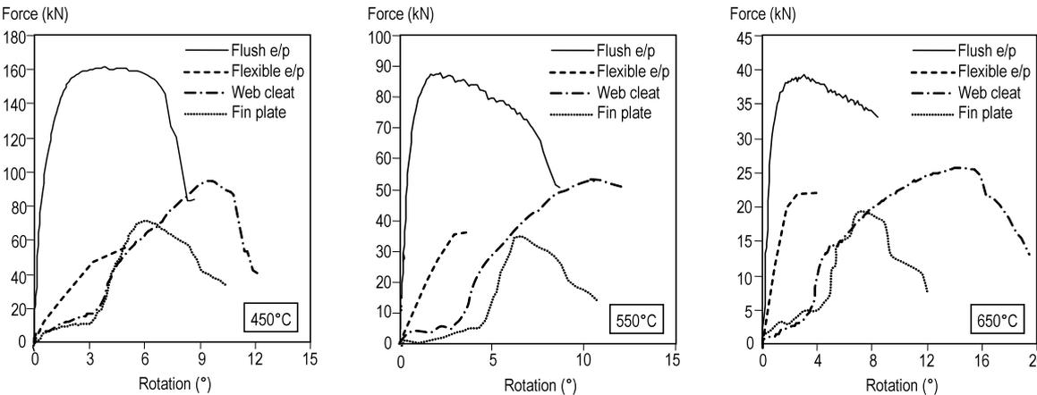
Figure 5. Behaviour of different connection types.
