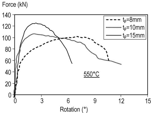
Figure 3. Effect of endplate thickness.
