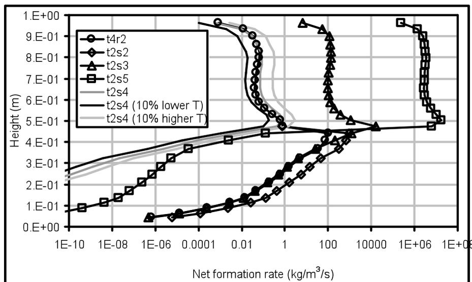
Figure 2. Predicted net CO formation rates against height at the front of the RSE [Key: Westbrook & Dryer (1981) Table 4 row 2 (t4r2) and Table 2 sets 2-5 (t2s2-5)].
