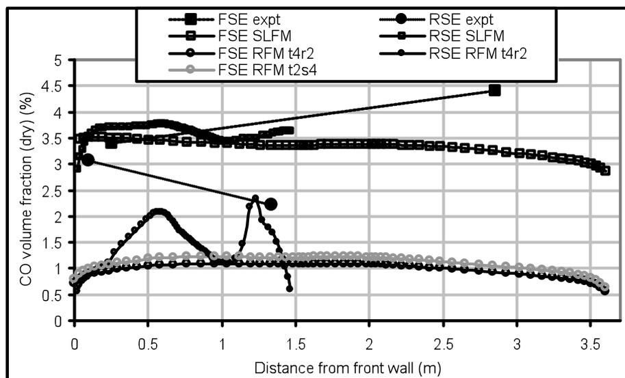
Figure 1. CO yield profiles in the hot layer [Key: experiments (expt), steady laminar flamelet model (SLFM), rate flamelet models (RFM) with kinetic mechanisms from Westbrook & Dryer (1981) Table 4 row 2 (t4r2) and Table 2 set 4 (t2s4)].
