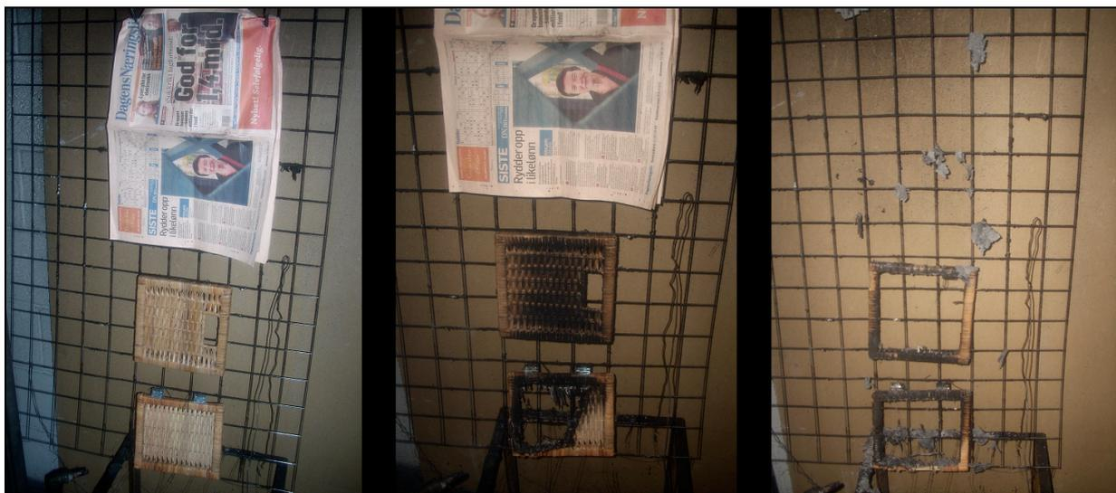
*Figure 9: From left to right: test specimens before the test, test specimens after the test at 15.9 vol%, test specimens after the test at 20.9 vol%.*
