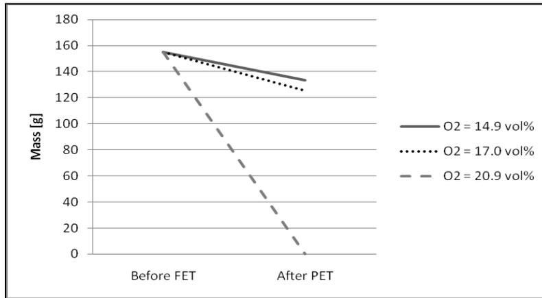
Figure 6: Test specimen mass (before FET and after PET) of the ignition test of PP (vertical configuration).
