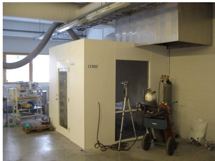
*Figure 2: The test enclosure. The door and the observation windows allow observation of fire tests from three different sides.*
